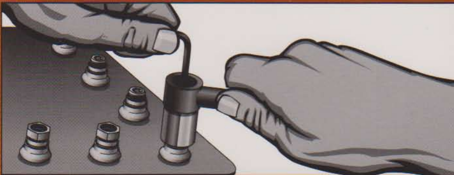
Shown: Installing the Hi-Lok® fastener with the "Roller Clutch" wrench.
